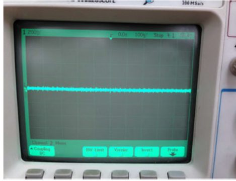
(b) Synchronization error for unidirectional cosine function based coupling. Vertical scale is 200 mV/div., horizontal scale is 100 \mu s/div.
